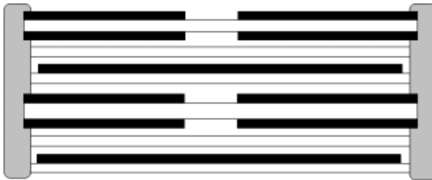
Double-sided metallized electrodes with internal series connections
