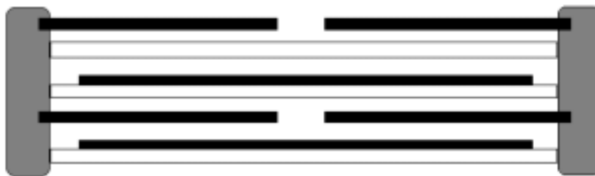
Extended foil electrodes and metallized film with internal series connections
