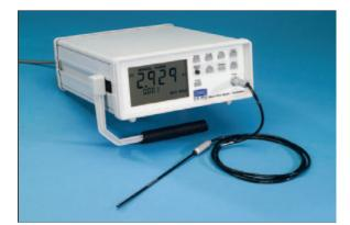
The Model 6010 Hall-effect Gauss/Tesla-Meter features F.W. Bell's exclusive Dynamic Probe Correction, along with temperature compensation and allows measurements up to 300 kG with a basic accuracy of 0.25%. Key features include Peak Hold, Max/Min Hold, Auto Zero, Auto Range, Relative Mode and Temperature measurement. The Model 6010 allows the user to select Gauss, Tesla or Ampere/Meter readings. The Model 6010 also features a corrected analog output (± 3 V Full Scale for each range),
