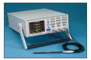
The F.W. Bell 7000 Series Gauss/Tesla-Meters lead the way for Advanced Hall Effect Magnetic measuring technology. The easy-to-use front-panel programming feature incorporates the latest in user control operations. The 7000 Series instruments are capable of simultaneously measuring and displaying seven different parameters per channel – 27 total parameters for the 7030 three-channel model.
