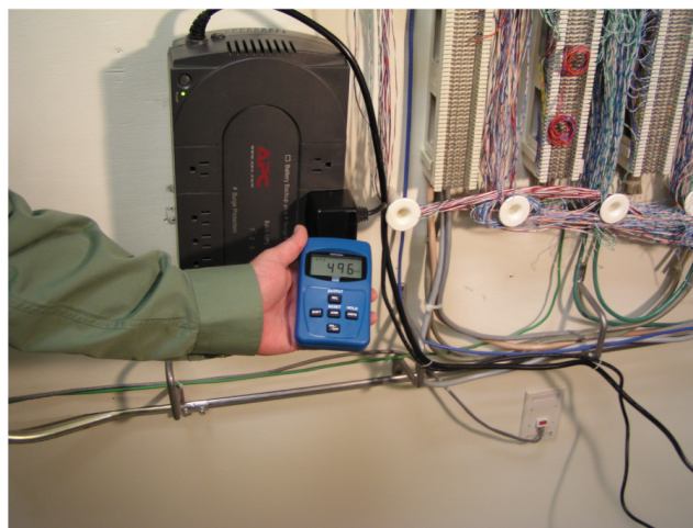
Example of ELF radiation located in a typical telephone switching room and how to detect it
