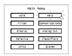
To enter a sub-menu, position the "pointer" over a "button" and press the ENTER key. To return to the main menu, press the MENU key.
