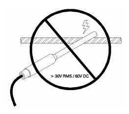
Figure 4-1 Probe Electrical Warning
