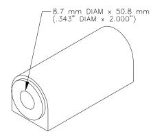
Figure 2- 3 Zero Flux Chamber
