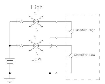
Figure 6-7 Example Circuit for Classifier Outputs
