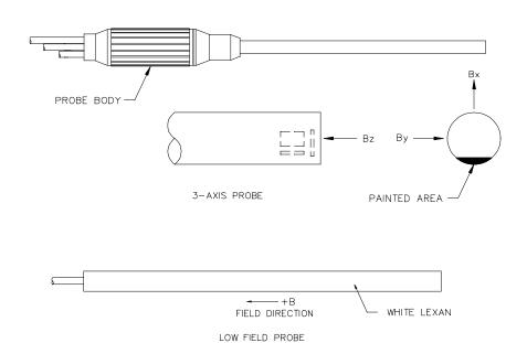
Figure 3-2 Hall Probe Configurations
