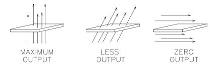
Note: The probe is calibrated and specified with flux lines passing perpendicularly through the Hall effect sensor.
