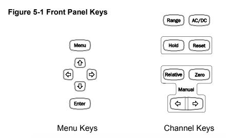
Each key features a back-light that will illuminate indicating that it is active. For example, if channel 1 is disabled, its set of keys will not be illuminated. In some instances, certain keys will flash indicating that a particular function is enabled or that some condition requires attention.
