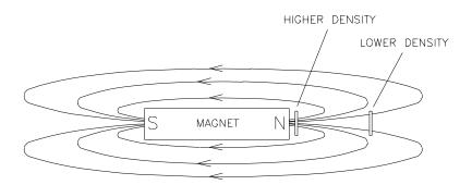
5) Flux density can vary considerably across the pole face of a permanent magnet. This can be caused by internal physical flaws such as hairline cracks or bubbles, or an inconsistent mix of materials. Generally the sensitive area of a Hall effect sensor is much smaller than the surface area of the magnet, so the flux density variations are very apparent. Figure 6-10 illustrates this situation.
