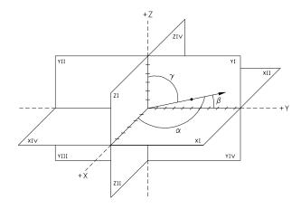
Figure B-4 Vector Angles in a Three-Dimensional System
