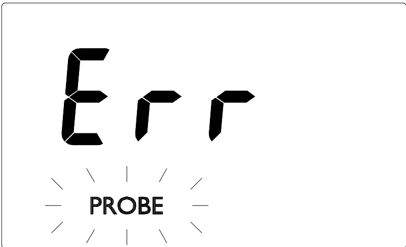
Figure 3-5 Missing Probe Indication
