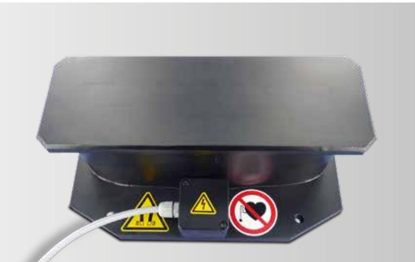
The Portable Demagnetizing Device **LIST-MAGNETIK HE-2** can be used either mobile or stationary, as required. The portable device demagnetizes machine parts, tools, rotary parts, cutting plates and much more. It has a 230 V AC connection and produces an alternating magnetic field of 50 Hz with sufficient field strength for the demagnetization of alloyed steels.
